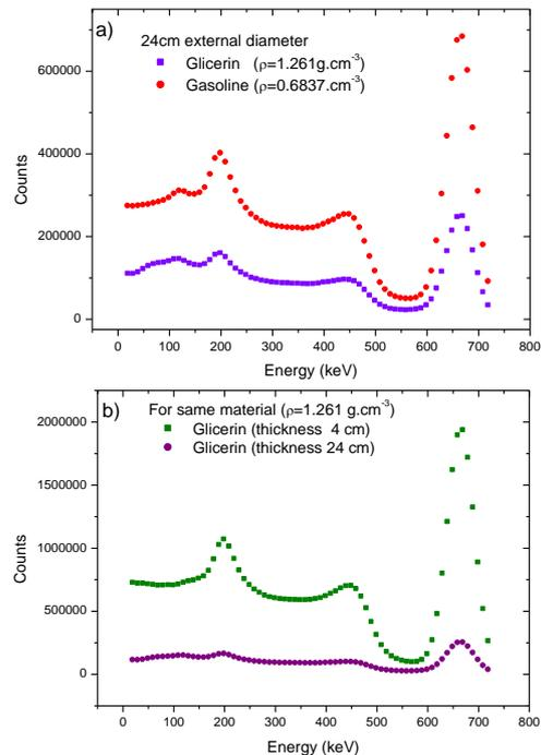
Figure 2. The PHD for: a) two different materials for the same thickness absorber; b) two different thickness of absorber for the same materials.
