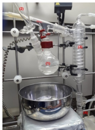
Figure 1: Glass device for synthesizing the radioactive methyl bromide tracer consisting of four parts: (1) Synthesis vessel, (2) Dropping funnel and (3) Friedrichs condenser.
