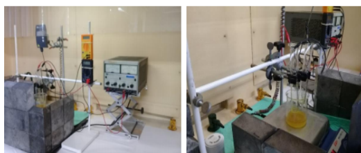
Figure 1. Representation of the experimental apparatus of electrochemical synthesis for organic phase labeling with bromine-82
