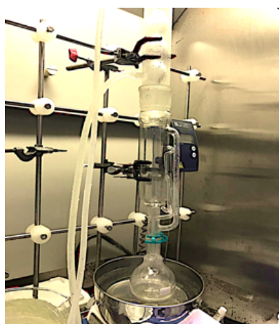
Figure 1. New synthesis apparatus for production of the radiotracer CH 3 I labeled with radioiodine.
